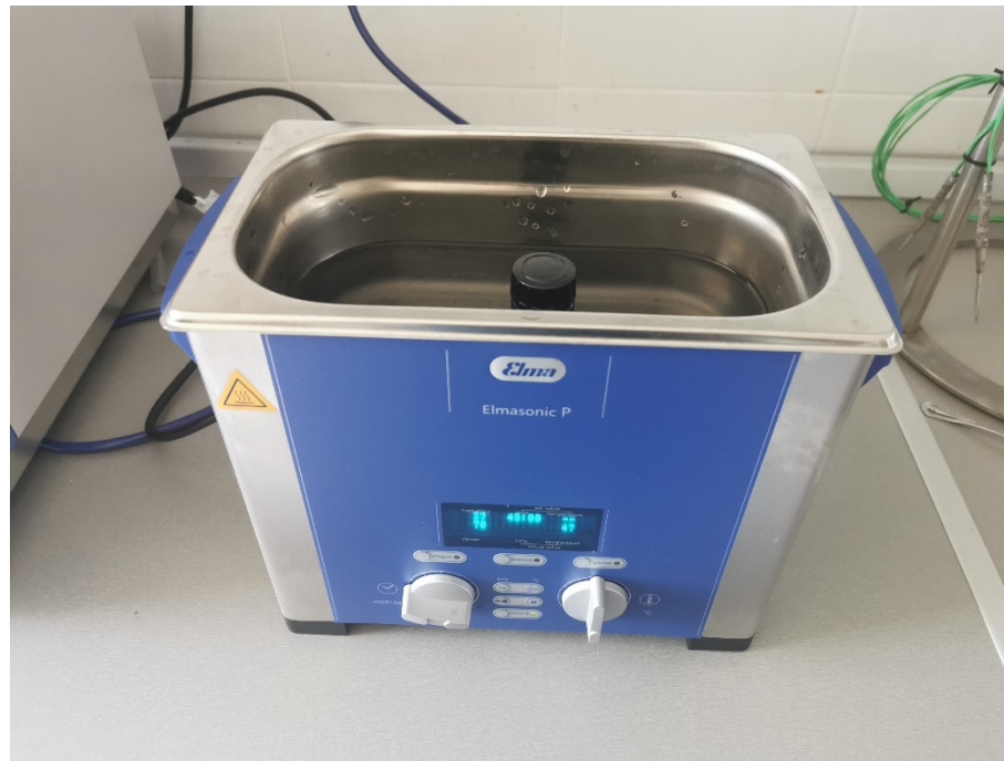
Ultrazvučno kupatilo, model Elmasonic P (Elma, Germany) 45 min, 37 kHz
